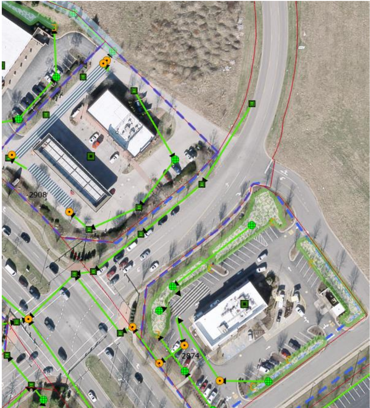
Example of stormwater, SCM, and SCM indicators features in GIS. SCM sites are color coded by development phase (yellow: planning, red: construction, green: post)
