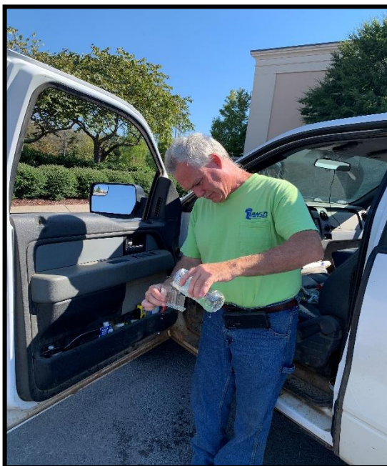
9/29/2021 - Bruce Ross checks for chlorine in flow detected in drainage system at Stones River Mall. Determined to be groundwater. Flow unrelated to wash water.
